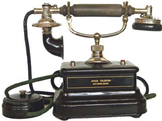
The design dates back to the usual Kirk desk telephone from 1909, but the electronic circuit and operation are different. This set has been used in Aalborg, Denmark. It is a part of a system using so-called alternator ringing. The alternator ringing system was mainly used by larger companies with many extension telephones connected to a switchboard. When the red button is pushed the alternator sends out the
